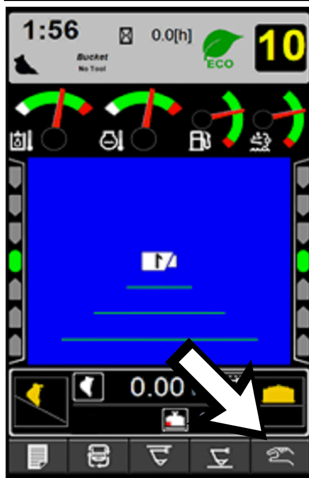
Illustration 148 g03874649 Multi-Information Area with Button to Select Manual Mode
